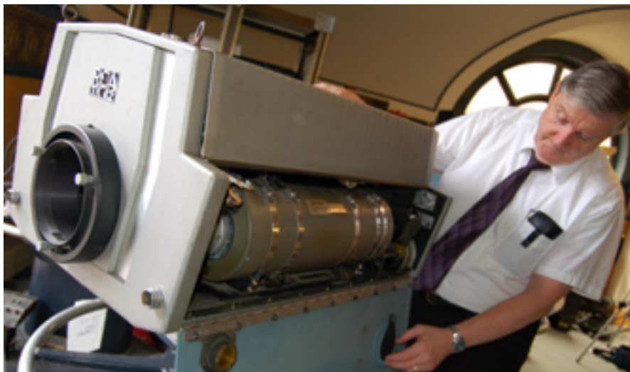
A TK 42 colour camera sans lens. Three 1" inch Vidicons and a 4 ½" inch Image Orthicon tube combined. Not a happy mix. 'Muddy' flesh tones apparently
